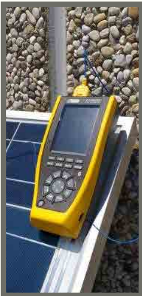
Temperature measurement on solar panels. The practical magnetized Multifix accessory allows you to work hands-free.
